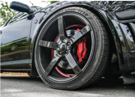
Tarox brakes on the Gen I have a strong bite but they tend to fade after hard use.
