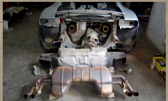
The heat shield and standard exhaust are out
