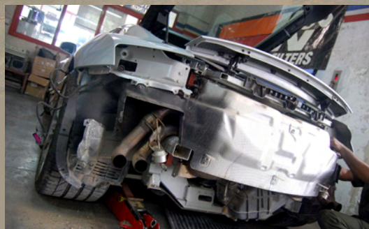
Removing the rear bumper and tail lights
